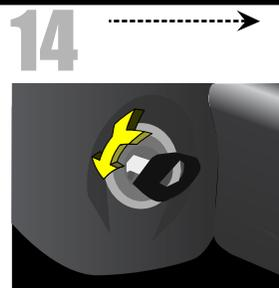
14 Turn off engine, and remove sensor head.
