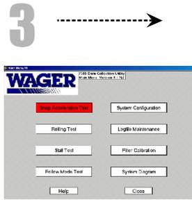
3 On the main menu, Select the "Snap Acceleration Test" button.
