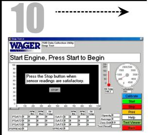
10 When oil temperature and RPM readings are satisfactory, press "Stop" button, Pre-snap test will automatically begin.
